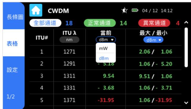
The screenshot shows a mobile application interface for CWDM monitoring. At the top, there are three status indicators: '全部通道 18' (All Channels 18), '正常通道 14' (Normal Channels 14), and '異常通道 4' (Abnormal Channels 4). Below these is a table with the following data:
