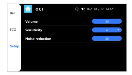
Directly tap the blue button next to Volume first. Second, short press [ ] key or directly tap [+] on the screen to turn up the volume or short press [ ] key or directly tap [-] on the screen to turn down the volume. And then short press [ ] key or directly tap [ OK ] to confirm the setting. Short press [ ] key or directly tap [ Cancel ] to discard it.
