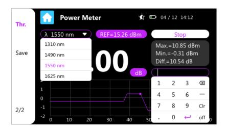
Input the value of the threshold and then directly tap [  $\leftarrow$  ] on the screen.
