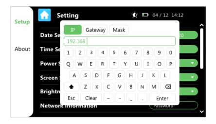
Directly tap [IP], [Gateway] or [Mask] on the screen, fill with the details in the text field, and then tap [Enter] to confirm it.
