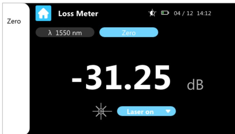
2. The value displayed on the screen is the loss value of optical fiber.
