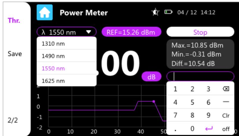
Input the value of the threshold and then directly tap [ **↩** ] on the screen.
