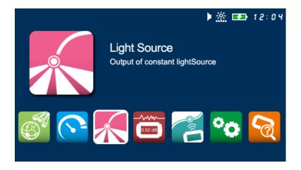
Short press [ - ] key to enter into the main display of optical light source.
