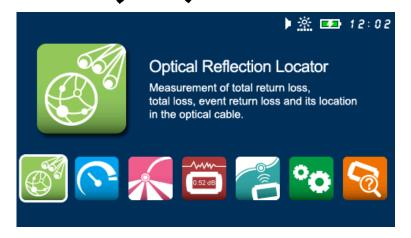
Short press [ ] key to enter into the home screen of optical reflection locator.
