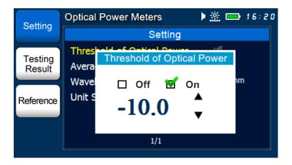
Short press [ ] or [ ] key to enable the threshold of optical power to turn ott.
