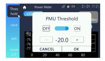
2. Short press [ ], [ ], [ ] or [ ] key to move the white dashed box to OFF or ON, and then short press [ ] key to confirm it or directly tap [ OFF ] or [ ON ] on the screen.
