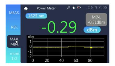
] on the screen can be switched by short 2. The value in [ pressing [ F3 ] key or directly tap [ MAX. MIN. ] on the screen.  $MIN. \rightarrow MAX. \rightarrow MAX.-MIN.$
