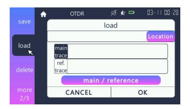
2. Directly tap [ main / reference ] on the screen to select main trace or reference trace and then short press [ • ] key or directly tap [Location] to select the saved trace. Directly tap [OK] to open it or [CANCEL] to cancel it.
