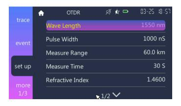
Short press [ ♠ ], [ ♦ ], [ ◀ 2. 1 key to ] or [ select the desired wavelength, and then short press the setting.
