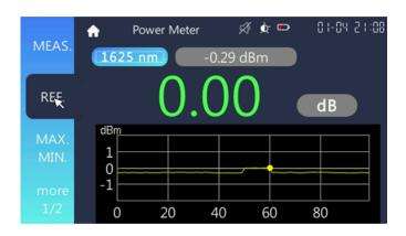
Connected to another optical fiber to be tested with light source, 2. the value displayed in the middle of the screen is the difference between the current measured optical power value and the reference value.
