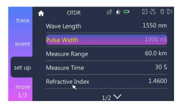
2. Short press [ ], [ ], [ ] or [ ] key to select the desired pulse width, and then short press [ ] key to confirm it. Short press [ ] key to discard the setting.
