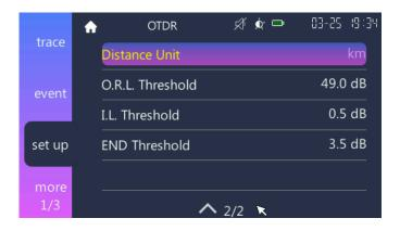
Short press [ ], [ ], [ ] or [ ] key to select the unit, and then short press [ ] to confirm it. Short press [ ] key to discard the setting.
