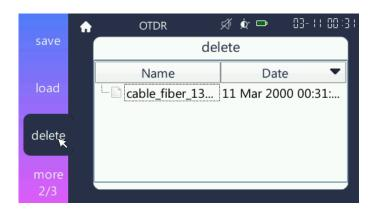
] or [ ] key to move to the files to be deleted, and then short press [ - ] key to delete it. Directly tap the files to be deleted on the screen and then tap delete ] on the screen to delete it.
