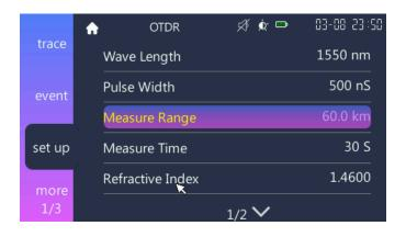
2. Short press [ ], [ ], [ ] or [ ] key to select the desired distance, and then short press [ ] key to confirm it. Short press [ ] key to discard the setting.
