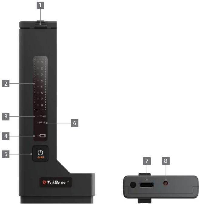
1 RJ45 port 2 Line sequence indicator light 3 Hunt function indicator 4 Low battery indicator 5 Switch off/Function switch button 6 Sequencing function indicator 7 Type -c port 8 Charging light
