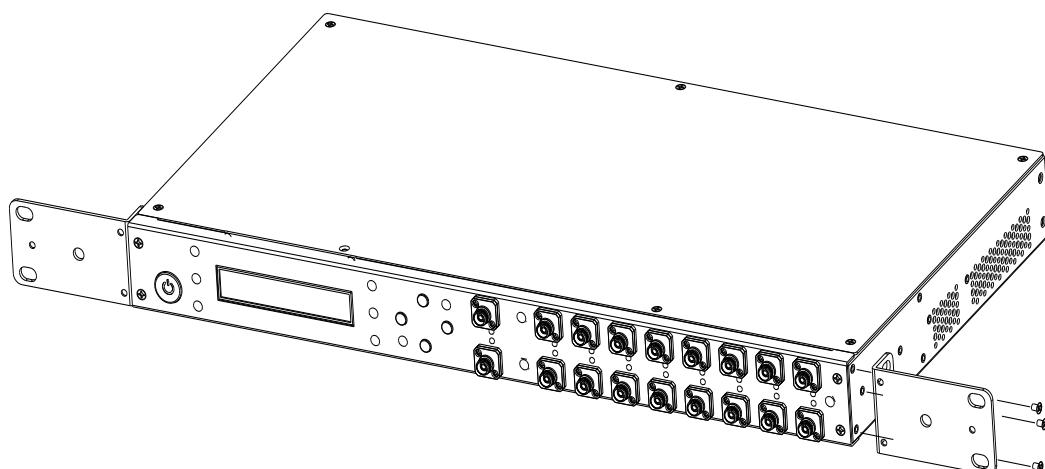
2. Align the screws on the mounting ear with the holes on the rack to position the equipment and use screws to fix the equipment to the rack.
