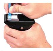
Turn the fiber-optic connector end-face to face one of the slot and slowly slide the connector down.
