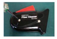
3 Use a flat screwdriver or a coin to tighten the screw
