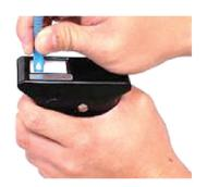
Turn the fiber-optic connector end-face to face one of the slot and slowly slide the connector down.
