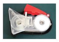
2 Remove the used cartridge and insert a new one properly
