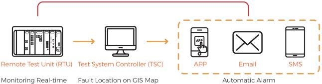
Monitoring Real-time Condition of Optical Fiber Fault Location on GIS Map Comprehensive Info & Analysis
