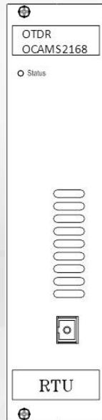
High Pass Filter (HPF) must be installed along with Optical Time Domain Reflectometer (OTDR). High Pass Filter (HPF) will filter out transmission signal in the structure of In-Line Monitoring or self-emitting light source from Light Source Unit (LSU) in the structure of Off-Line Monitoring in order to ensure the service life of Optical Time Domain Reflectometer (OTDR).
