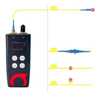
1. Fiber identification & End-to-end continuity tests
