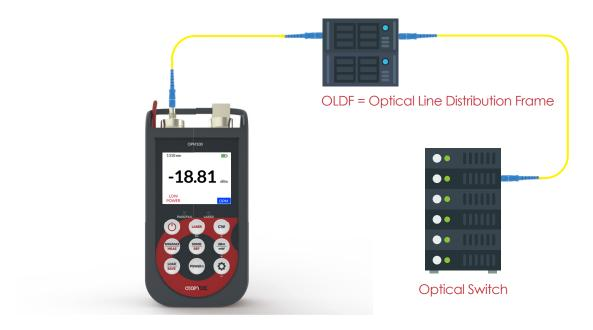
2. Optical Loss Measurement Performing with OLS to measure optical power to calculate optical loss
