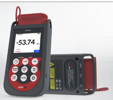
Ascentac OPM120 Series, Optical Power Meter, provides high accuracy for optical power measurement in fiber-optic network. It has a wide dynamic range from +6 to -70dBm or +26 to -50dBm. Offering seven calibrated wavelengths (850nm, 1300nm, 1310nm, 1490nm, 1550nm, 1625nm & 1650nm) makes it ideal for both single-mode and multi-mode fiber testing. Furthermore, its wavelength can be automatically selected when it is paired with Ascentac Optical Light source (OLS200).
