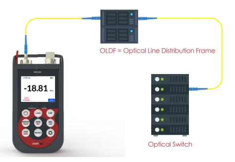
2. Optical Loss Measurement Performing with OLS to measure optical power to calculate optical loss
