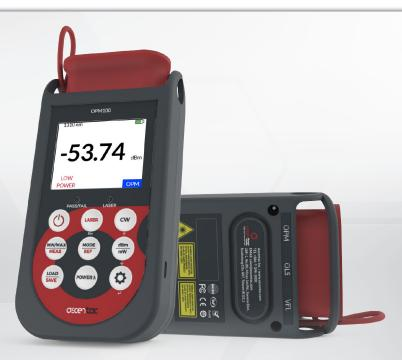
Ascentac OPM120 Series, Optical Power Meter, provides high accuracy for optical power measurement in fiber-optic network. It has a wide dynamic range from +6 to -70dBm or +26 to -50dBm. Offering seven calibrated wavelengths (85onm, 1300nm, 1310nm, 1490nm, 1550nm, 1625nm & 1650nm) makes it ideal for both single-mode and multi-mode fiber testing. Furthermore, its wavelength can be automatically selected when it is paired with Ascentac Optical Light source (OLS200).
