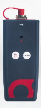
Ascentac VFL200 Series, Visual Fault Locator, is used for fiber identification or troubleshooting. It can help technicians to diagnose faults in optical fibers, including fiber damages or breaks, improperly attached fiber connectors, bending, and so forth.
